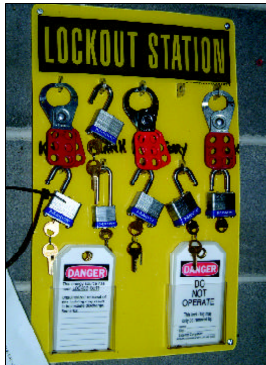
The use of lockout/tagout equipment during bin entry can prevent an engulfment incident before it gets started. Photo by Ed Zdrojewski.
